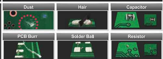
True 3D Foreign Material Inspection
